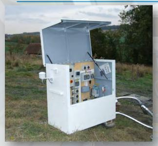
WJ can produce high quality data using our dedicated TRT unit which incorporates telemetric datalogging of flows, loop pressures, air and loop temperatures
